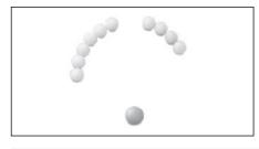
Easy-to-retrofit swivel angle limiter. After installation, the balls limit the swivel angle. Adjustable in steps of 14°. Material PA
