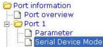
Modbus devices are commonly labeled as Master and Slave and therefore, the Serial Device Mode of the Modbus Gateway is also labeled as such modes, Master and Slave. When the port is set to Master, then the Ethernet will have to be set as Slave; vice versa, when the port is set to Slave, then the Ethernet will have to be set as Master. The following will explain the two configurations, (I) “Serial Device Mode” as “Slave” and (II) “Serial Device Mode” as “Master”.
