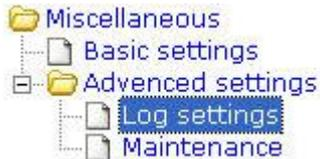
Enables and disables the Modbus Gateway communication logs. Enabling the communication log will increase resource consumption of the system, and therefore it is not recommended for units that are currently online. The default is to disable the communication logs. **It is recommended that the communication log only be enabled during non-online use for testing and debug purposes.**
