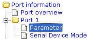
Parameter contains the following basic parameters for the port: Hardware Mode, Baud Rate, Data Bits, Parity, Stop Bits, and Flow Control.
