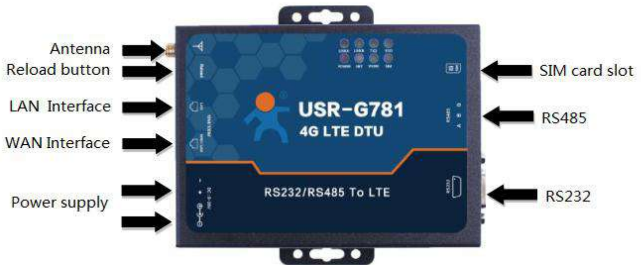
Figure 11 Hardware interface schematic diagram
