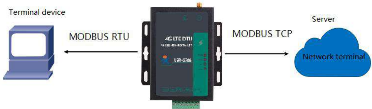
Diagram 15 Modbus protocol conversion schematic diagram
