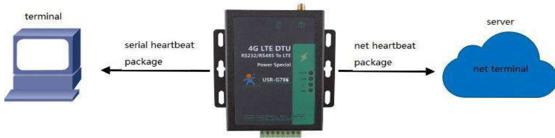
Diagram 10 Heartbeat schematic diagram
